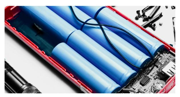
Lithium-ion batteries contain two electrodes (anode and cathode), a liquid electrolyte, and a separator, a semi-permeable barrier that isolates the anode and cathode from each other.
