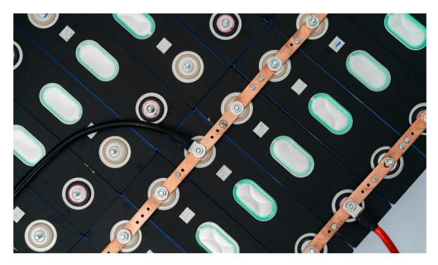
Battery manufacturers and automakers have been promoting a narrative implying that LFP, while storing less energy than NMC and NCA, is a "safe" option compared to higher energy chemistries, and is incapable of thermal runaway. This position is misleading at best.
